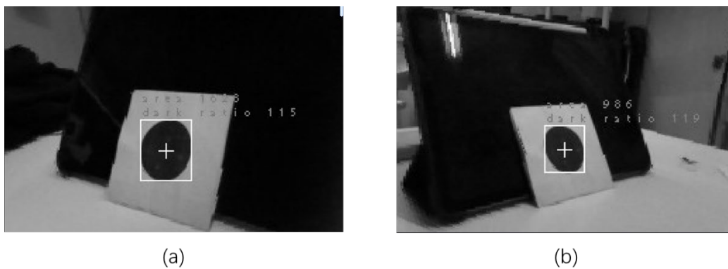
Figure 31. Recognition under severe perspective distortion. (a) Recognition at 35^\circ on the right. (b) Recognition at -40^\circ on the left.
