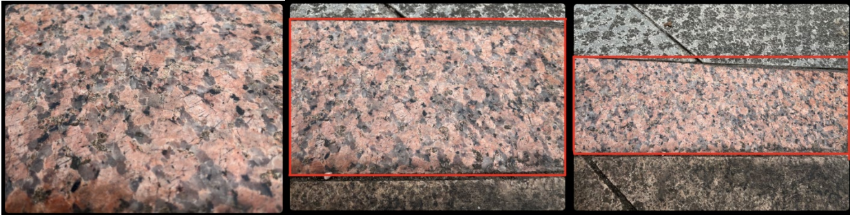
Figure 69. OpenMV installed at a height of 5cm, 15cm and 25cm.
