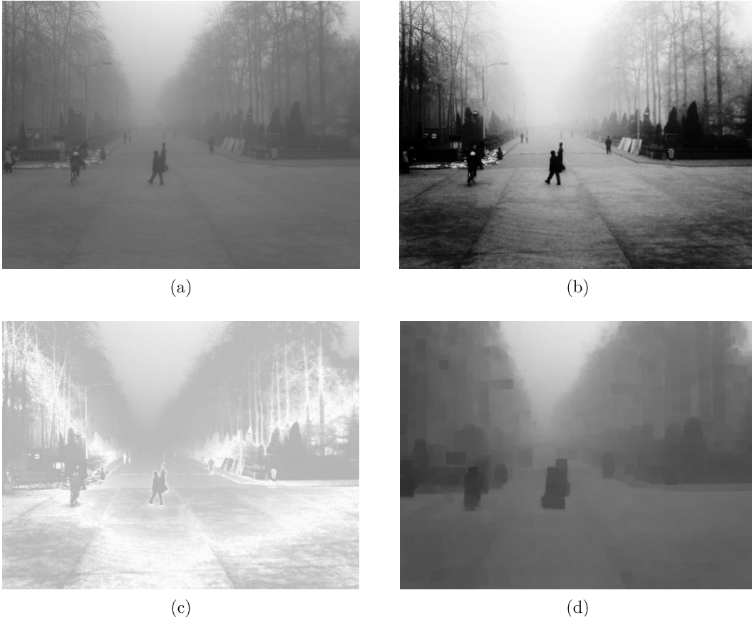
Figure 3. (a) The grayscale version of an original image. (b) Histogram equalised version of the grayscale image. (c) Dark channel generated by our proposed method. (d) The original dark channel. It can be observed that (c) and (d) are similar apart from the dilation in (d), and the main difference in this case is an offset.
