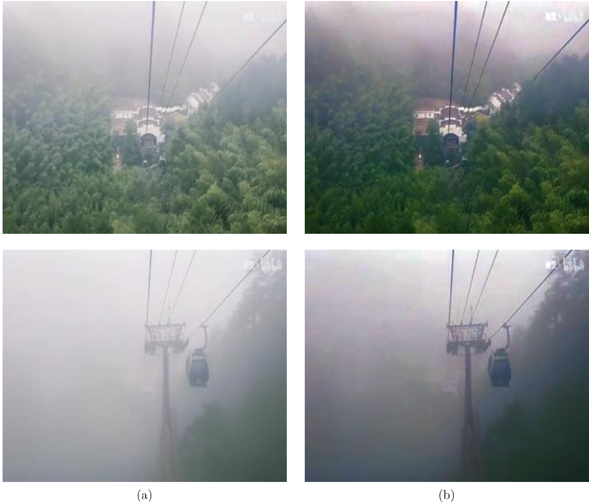
Figure 5. Dehazing performance of ST-MRF on a video in IEV2022 shot at the Yellow Mountain. Images in group (a) are frames from the hazed videos, and group (b) shows their dehazed counterparts. Images in group (b) shows higher contrast compared to image (a), as the illumination appears to be more uniform. Both frames in group (b) show very natural restored colour without unreasonably high saturations or semantically unexpected colours.
