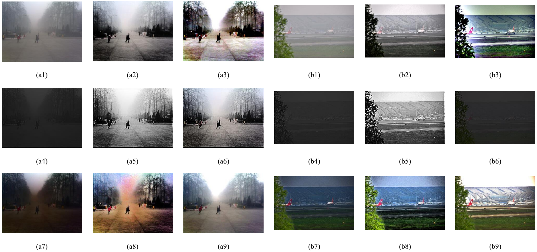
Figure 2-1. Comparison of different dehazing techniques on two hazy images (a) and (b) and two clear images (c) and (d), including (1) original image, (2) histogram equalisation, (3) Single Scale Retinex (SSR), (4) Homomorphic filtering on grayscale original images, (5) the previous technique followed by a histogram equalisation, (6) Homomorphic filtering on the value channel of the original image in the HSV colour space, (7) Dark Channel Prior, (8) Dark Channel Prior followed by a histogram equalisation, and (9) our proposed method. Our proposed method is good at restoring the colour information while dehazing, although it may not recover as much details compared to the original Dark Channel Prior.
